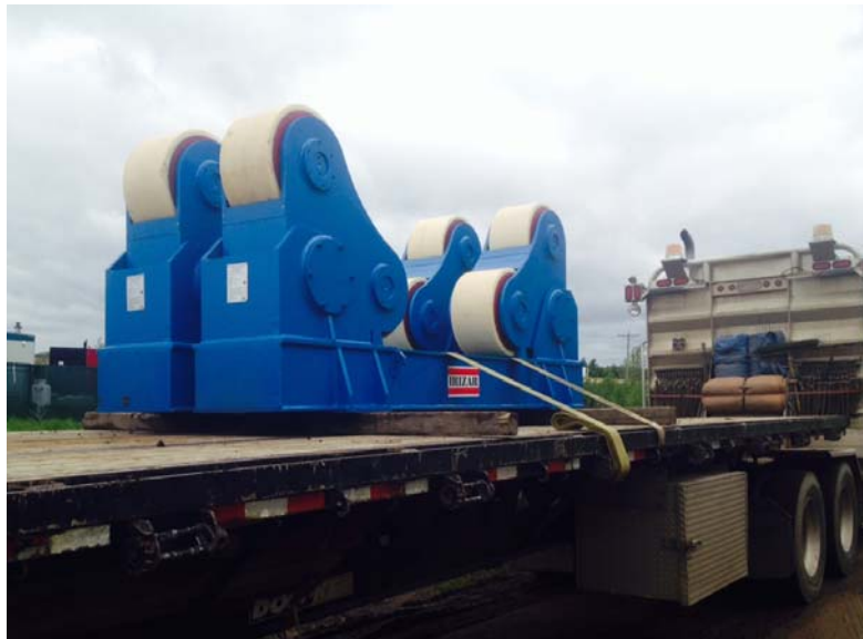
SAR 150 WITH POLYURETHANE WHEELS
