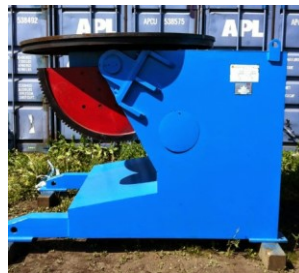
10 MT (22,000 #) @ 400 mm GC on Irizar Model WP 10 At Work in Edmonton, AB, Canada
