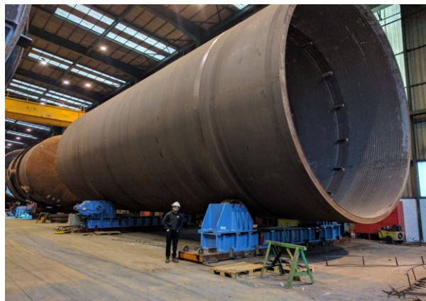
Irizar Welding Rotator Model WR 1200 Engineered in Canada. Load & Rotation Capacity: 1,200 MT At Work in the USA, Spain & China
