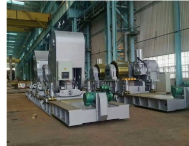
2500 MT, Irizar Anti-Drift Welding Rotator Model AD-WR 2500
