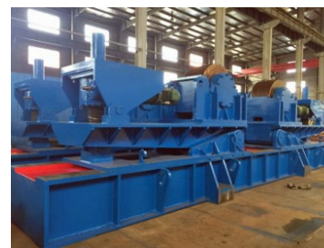
1600 MT Irizar Model Anti-Drift Idler IR 1600
