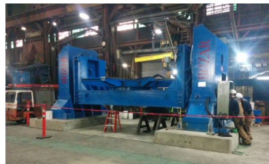
88,000 # @ 47.25" GC on Irizar Model CWP 40 At work Portland, Oregon, USA
