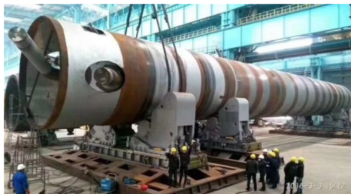
Anti-Drift Welding Rotator Model WR 3000 3000 MT load and rotation capacity
