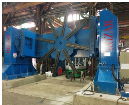
40 MT @ 1,200 mm GC on Irizar Model CWP 40 At work Portland, Oregon, USA
