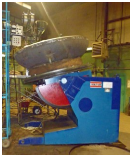
10 MT (22,000 #) @ 400 mm GC on Irizar Model WP 10 At Work in Edmonton, AB, Canada
