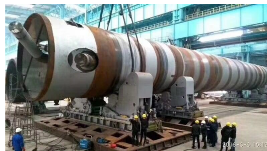
3000 MT, Irizar Anti-Drift Welding Rotator Model AD-WR 3000
