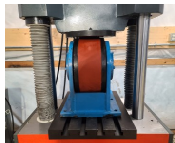
Welding Rotator's wheels tested on Irizar UTM
