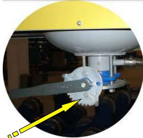
Outlet of recovery machine
