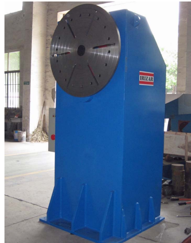
HEAD AND TAIL STOCK WITH FIXED HEIGHT CENTER ROTATION
